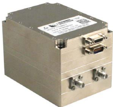
1. A tri-band transmitter can support S-, L-, and C-bands.
