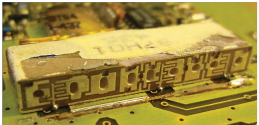
2. Shown is an example of a monoblock filter used in a 1994 Motorola handset.
