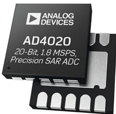
1. Model AD4020 is an example of a high-resolution ADC, at 20 bits. It samples analog input signals at 1.8 Msamples/s, but only consumes 15 mW from a +1.8-V dc supply at the maximum sampling rate. (Courtesy of Analog Devices)
