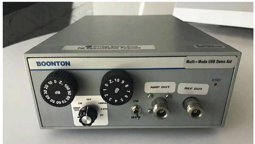
3. The demo aid is equipped with two output ports: REF OUT and AMP OUT.
