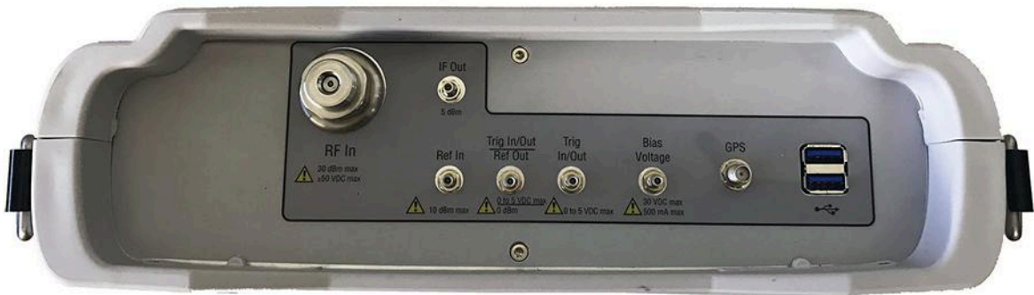
3. The intelligent design of the Field Master Pro MS2090A analyzers includes top-mounted connectors, protected by a recessed cavity.
