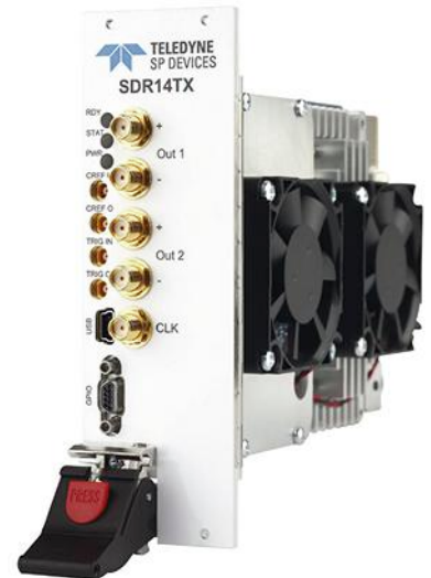
1. The modular SDR14TX arbitrary waveform generator (AWG) operates at sampling rates to 2 Gsamples/s and synthesizes output signals in the first Nyquist zone to 1 GHz and in the second Nyquist zone to 2 GHz. (Courtesy of Teledyne SP Devices)
