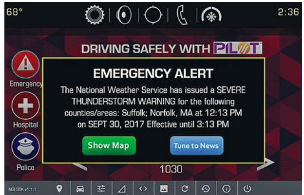
3. ATSC 3.0 enhances the concept of a digital dashboard by delivering audio, 4K video, text alerts, and other features to vehicle infotainment systems. (Source: NAB)
