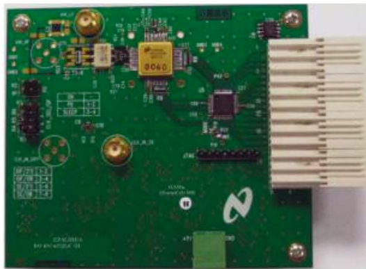
2. Evaluation boards can simplify the testing of high-speed ADCs like the 14-b model ADC14155, which operates at sampling rates to 155 Msamples/s and typical full-power bandwidth of 1.1 GHz for IF sampling. (Courtesy of Texas Instruments)
