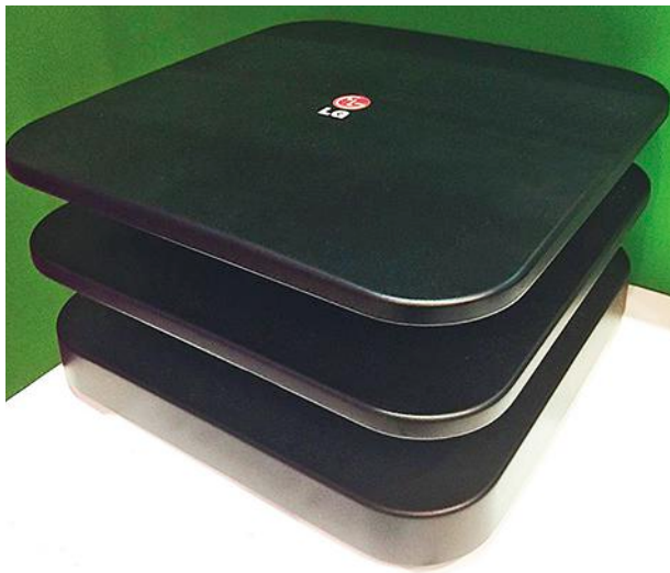
2. The LG Electronics ATSC 3.0 Smart Antenna combines the ability to receive OTA broadcast using an electronically-steerable antenna with an Ethernet interface to broadband to provide over-the-top content. An ATSC 1.0 tuner allows for backward compatibility. The combined signals are connected to a Wi-Fi router for distribution throughout a home. (Source: LG Electronics)
