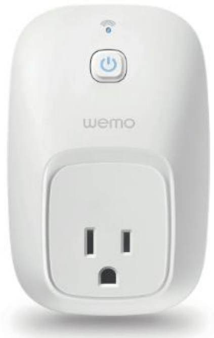
1. Some IoT devices are as simple as this WeMo switchable ac outlet, which enables remote control of home electronic appliances using an existing Wi-Fi network and a free downloadable application to run on a smartphone. (Courtesy of Belkin)
