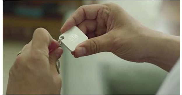
3. IoT-based object-location technology has been applied to a tracking device, thin enough to remain in a wallet, which can be found using a cellphone when lost. (Courtesy of Tile)
