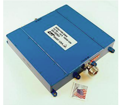
6. This miniature amplifier relies on GaN semiconductors to achieve 100 W CW output power from 13.75 to 14.50 GHz.
