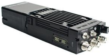
1. The modular MPU5 radios work with additional plug-in frequency modules to cover different frequency bands from L-band through upper-C-band frequencies.
