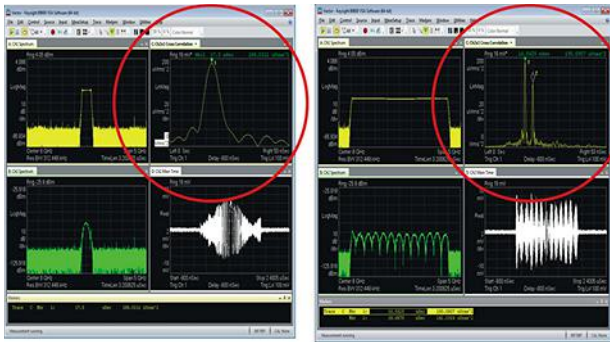
2. Looking at this bandwidth comparison, employing a 4-GHz bandwidth (right) enables two objects that are only 10 cm apart to be separated.
