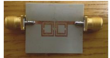
4. The second-order coupled SRR filter was fabricated on commercial circuit laminate material, with coaxial connectors attached for testing.
