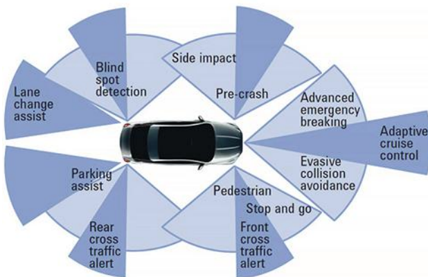
1. Shown are typical automotive mmWave radar applications and mounting locations.
