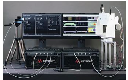
16. This 5G testbed for design validation can analyze the performance of a phased-array antenna in receive mode with a 3GPP NR signal in the presence of an unwanted interfering signal. (Courtesy of Keysight Technologies)
