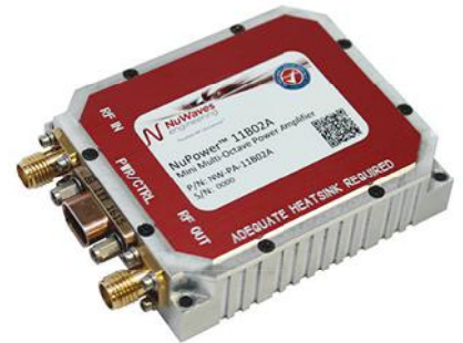
10. Efficient lightweight amplifiers like the NuPower 11B02A provide 10 W output power from 200 to 2600 MHz for UAV applications. (Courtesy of NuWaves Engineering)
