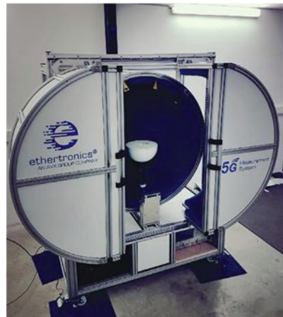
The mmWave 5G test chamber developed by Ethertronics can handle frequencies from 28 to 60 GHz.
