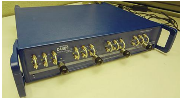
1. The C4409 4-port VNA is a member of Copper Mountain Technologies’ Cobalt series.
