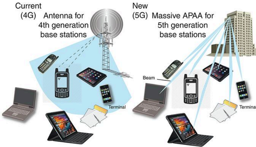
2. 5G massive MIMO requires active antennas with advanced beamforming technologies to direct narrow beams to stationary and moving targets in real time.
