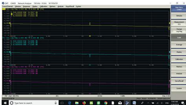
8. With the C4409, S_{21} , S_{31} , and S_{41} measurement data is displayed simultaneously.
