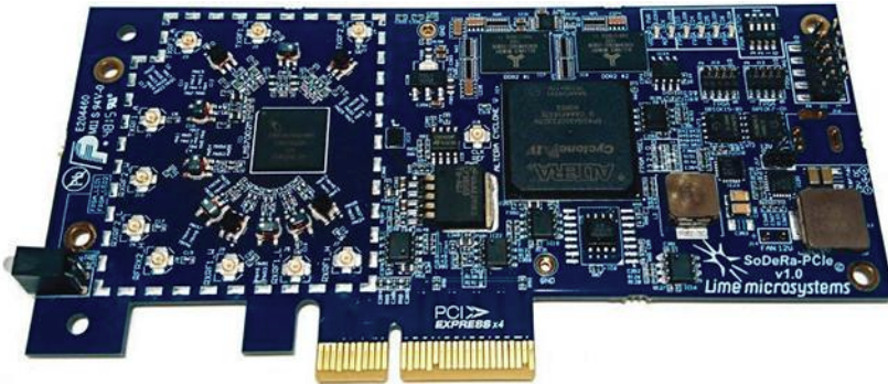
3. The LimeSDR SDR card is a key component of the LimeNET open-source small-cell hardware. (Courtesy of Lime Microsystems)
