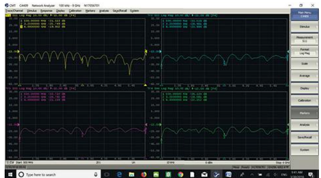
9. These measurement results represent the return loss at each of the power divider ports.
