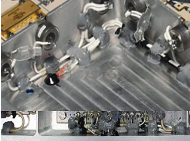
1. Signal routing in a test system is meant to avoid unwanted radiation of high-frequency signals that can be re-radiated within the system.
