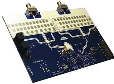
6. The iScan Radar Series modules are miniature radar system modules with options for 24-, 60-, and 70 GHz. (Courtesy of Colorado Engineering)
