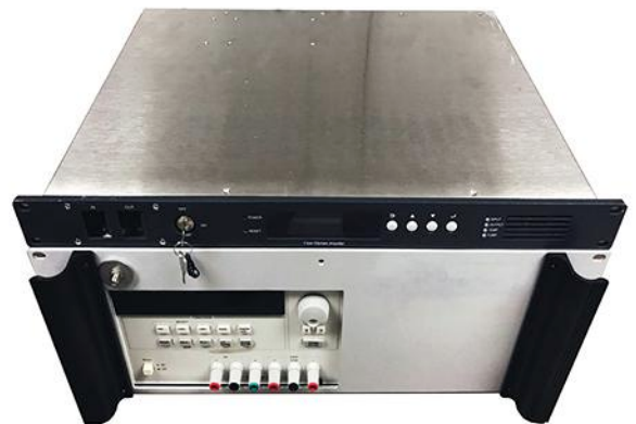
1. Shown in two views, this line of rack-mountable frequency synthesizers employs different techniques and technologies to trim phase noise at X- and K-band frequencies.
