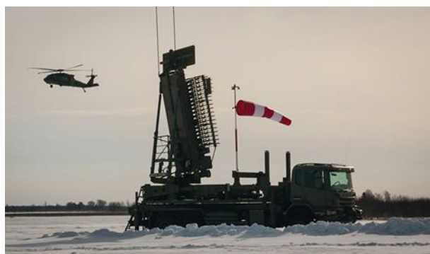
2. This is the TPS-77 MRR in Latvia during a site-acceptance test earlier this year. (Courtesy of 22nd Mobile Public Affairs Detachment)
