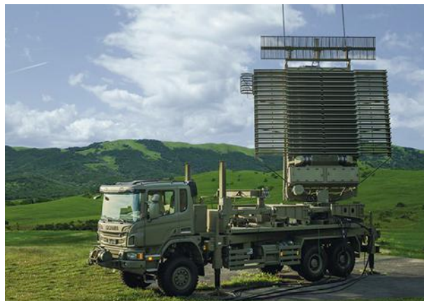
1. Here, the TPS-77 MRR is mounted in a truck in the deployable mobility configuration. (Courtesy of Lockheed Martin)
