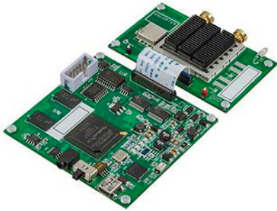
5. This 2.45-GHz kit makes it easy to get started with SDR technology. (Courtesy of Ancortek)
