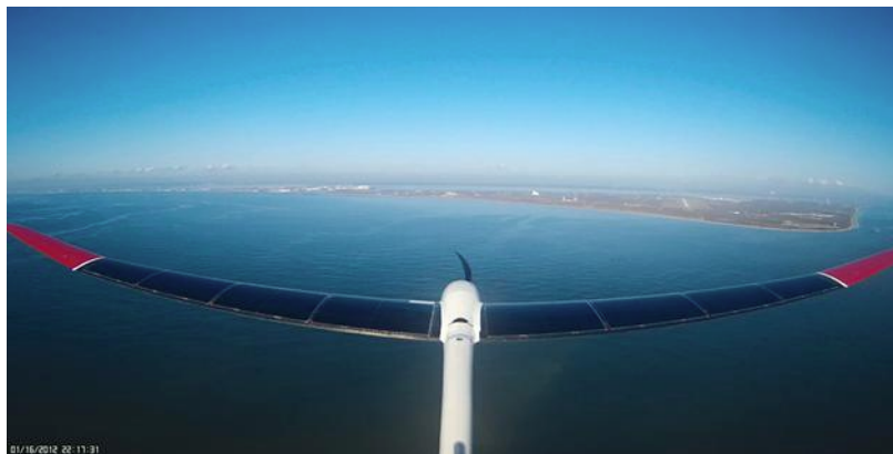
Solar Soaring is a combination of techniques applied by the NRL to extend the flight times of UAVs. (Courtesy of the Naval Research Laboratory, www.nrl.navy.mil )
