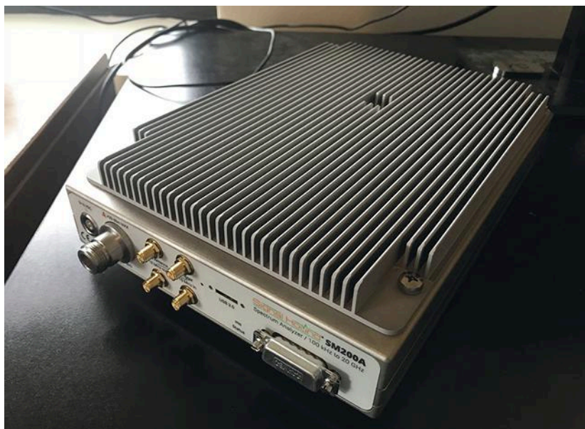
1. The SM200A is a 20-GHz spectrum analyzer and monitoring receiver.
