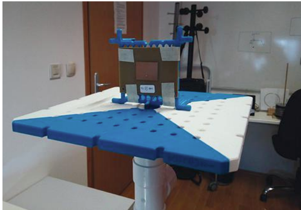
9. This test setup on the RMS measured the 2.45-GHz WLAN microstrip patch antenna.
