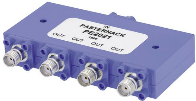
4. Pasternack's PE2021 4-way Wilkinson power divider operates from 7 to 12.4 GHz and handles 10 W of input power (CW).
