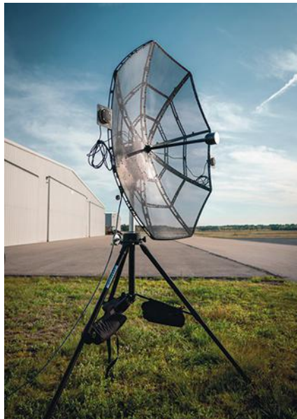
This portable antenna system uses interchangeable antenna feeds for operation at S-, L-, and C-band frequencies. (Courtesy of Persistent Systems, LLC, www.persistentsystems.com )
