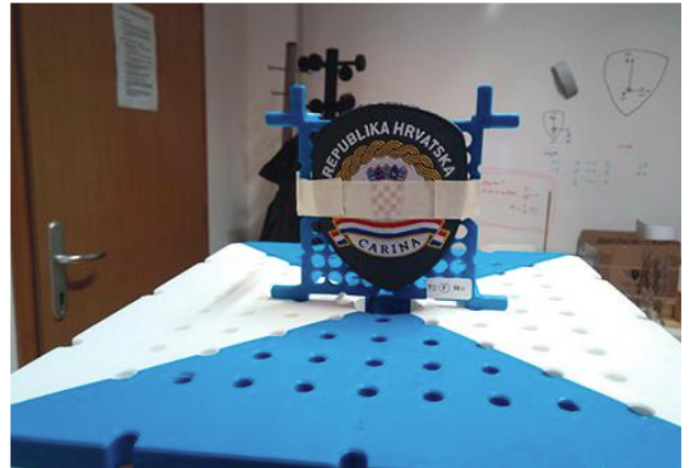
11. This is a prototype wearable sleeve-badge antenna being developed with the help of the RMS tester.
