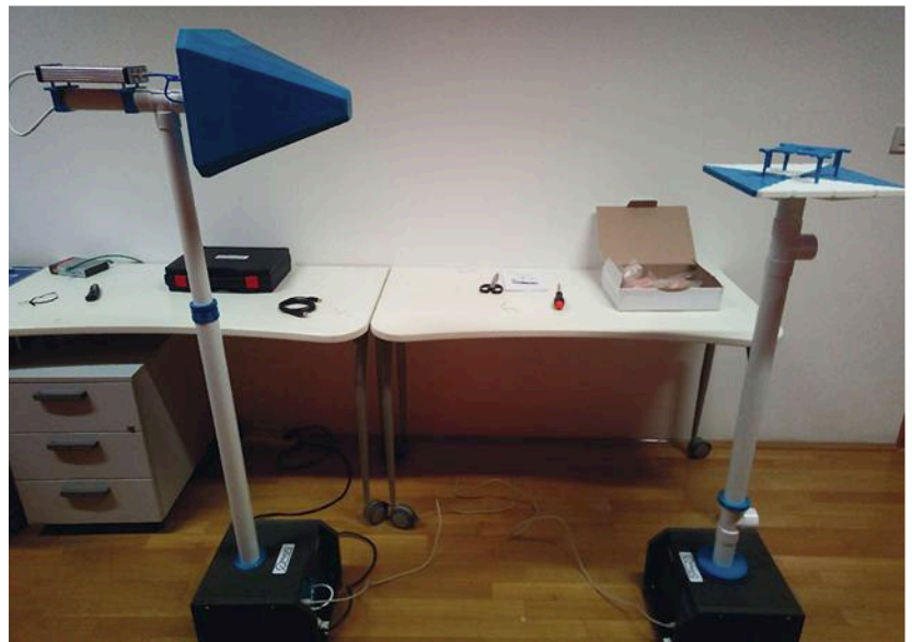
1. This is how the MegiQ Radiation Measurement System (RMS) appears when it's fully assembled and ready for testing antennas.
