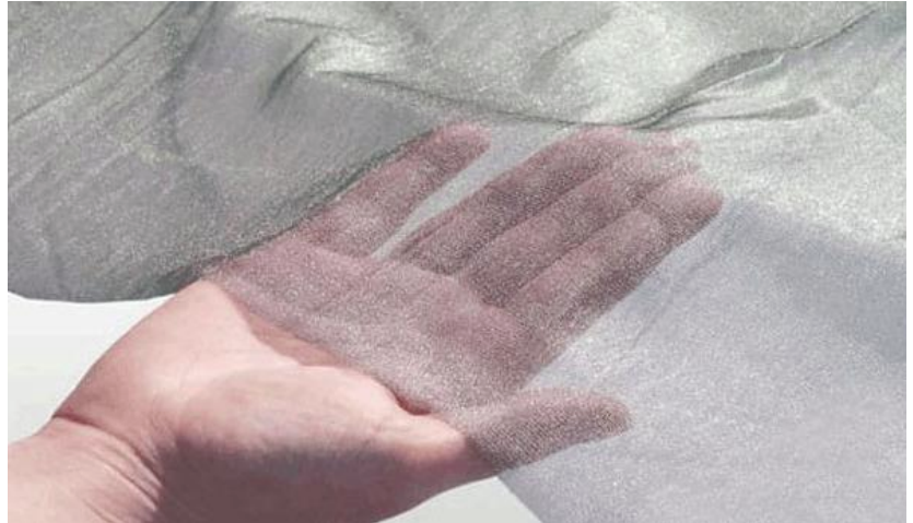
1. Lightweight silver/polyamide mesh shielding materials are capable of 50 dB or more shielding. (Courtesy of AaroniaUSA)
