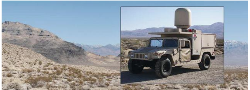
1. The AN/TPS-78 is a transistorized, transportable S-band air-surveillance radar system that uses Doppler processing for long-range detection. (Courtesy of Northrop-Grumman)
