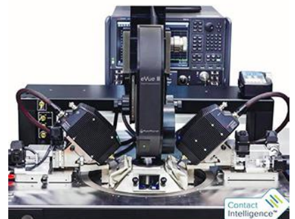
2. This autonomous RF measurement solution can perform autonomous calibrations and measurements of RF devices over multiple temperatures.
