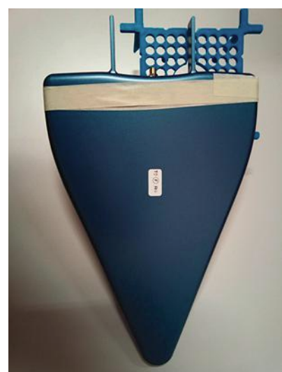
6. This commercial log-periodic antenna was tested on the RMS from 700 MHz to 6 GHz.
