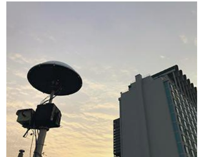
The AARTOS Drone Detection System, shown here in a Singapore application, is capable of detecting and tracking UAVs and their users.
