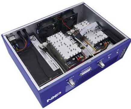
2. The RFEL24-500 lab box contains two RFEM24-250 modules plus other integral series devices.
