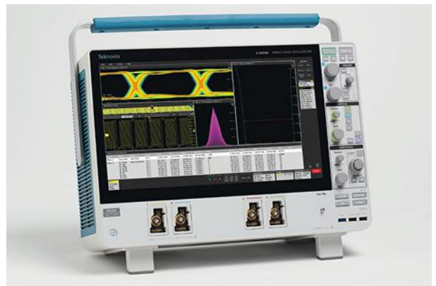
The 6 Series MSO oscilloscopes offer bandwidths as high as 8 GHz along with 25-Gsample/s sample rates.
