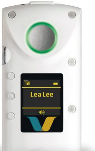
2. Healthcare monitoring and reporting are of growing importance for wearables such as this compact communications badge operating within the Wi-Fi band. (Courtesy of Vocera)
