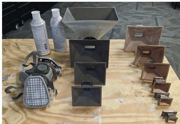
2. A variety of different antenna types and sizes can be formed by 3D-printing plastic foundations that are subsequently coated with conductive paints.
