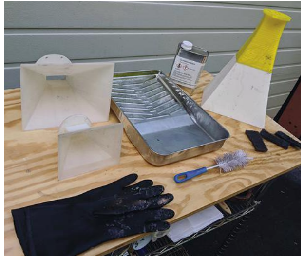
5. These are the tools for smoothing a 3D-printed antenna surface outdoors.
