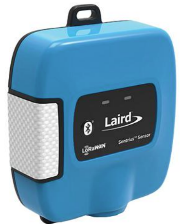
2. Laird's Sentrius RS1xx LoRa-enabled sensor is a battery-powered, long-range integrated sensor platform that leverages the benefits of LoRaWAN and Bluetooth Low Energy (BLE) connectivity.
