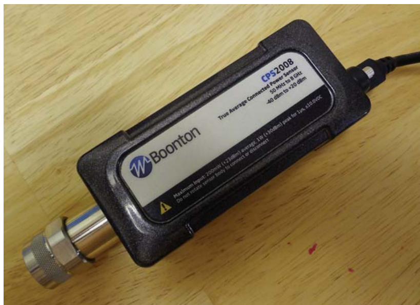
1. The CPS2000 Series power sensor covers a frequency range of 50 MHz to 8 GHz.
