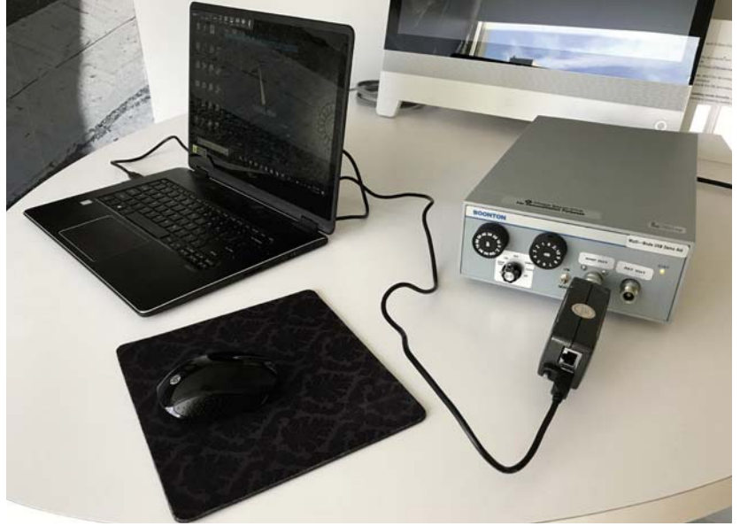
2. In this setup, a CPS2000 Series power sensor is measuring a signal from a Boonton demo aid.
