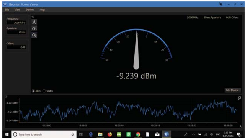
3. Here, the Boonton Power Viewer software displays a power measurement reading of -9.239 dBm.
