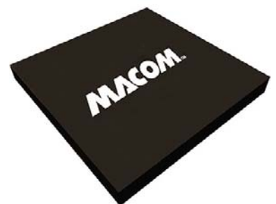
1. The MASW-011102 SPDT switch, which operates from dc to 30 GHz and maintains 1.8 dB of insertion loss across the entire band, comes in a PQFN package as shown here.
