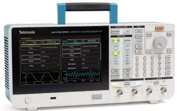
1. The AFG31000 Series of arbitrary function generators (AFGs) combine precise signal-generation power with an intuitive user interface for ease of control.
