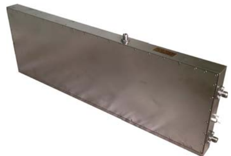
1. This module provides common stable LO signals for the mmWave frequency down-conversion modules.
