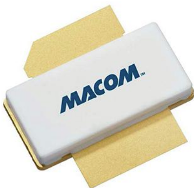
1. This hermetic package holds a high-power, +50-V dc Si bipolar transistor capable of 350 W pulsed output power from 1025 to 1150 MHz for Mode-S aviation radar transmitters. (Courtesy of MACOM)
