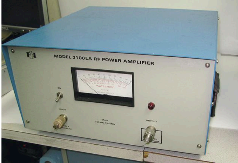
2. Model 3100LA is a robust Class A PA with high linearity from 250 kHz to 150 MHz. (Courtesy of ENI)
