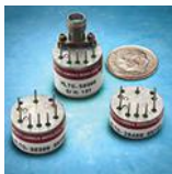
MLTO-series TO-8 Oscillators 2 to 16 GHz
