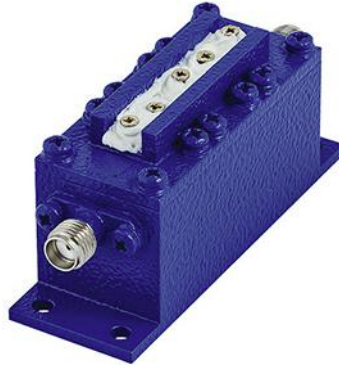
1. The ZVBP Series of compact cavity bandpass filters covers passbands to 15 GHz and stopbands to 20 GHz. (Courtesy of Mini-Circuits)
