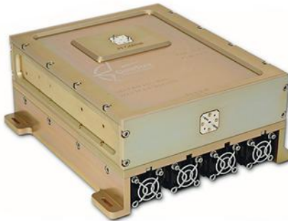
11. This GaAs-MMIC amplifier is designed for pulsed and CW signals at W-band frequencies from 92 to 96 GHz. (Courtesy of QuinStar Technology)
