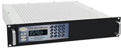
13. The model 50PSA-101-XX programmable phase-shifter assembly has a phase range of 0 to 358.6 deg. in 1.4-deg. steps for center frequencies from 1.5 to 3.0 GHz. (Courtesy of JFW Industries)
