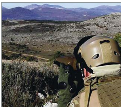
1. The JIM Compact IR binoculars measure the distance to a target as well as the motion of the target and calculate a bullet's flight time to improve sniper effectiveness. (Courtesy of Safran Electronics & Defense)
