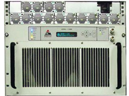
The APRA-S2500A is a GaN-based S-band SSPA capable of 2500 W pulsed output power from 2.7 to 2.9 GHz. (Courtesy of Advantech Wireless)
