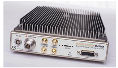
15. Model SM200A is a real-time spectrum analyzer with 110-dB dynamic range from 100 kHz to 20 GHz that can be used as a monitoring receiver. (Courtesy of Signal Hound)
