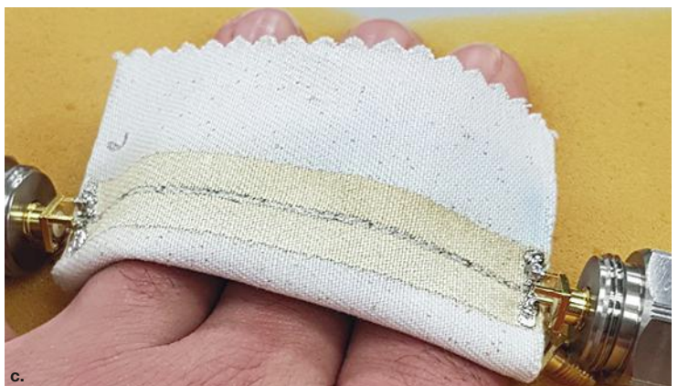
7. The 80-mm transmission lines were tested with a hand underneath (a), an insulation layer between the hand and the lines (b), and another line folded underneath and a hand below (c). (See Figure 6 for the results).
