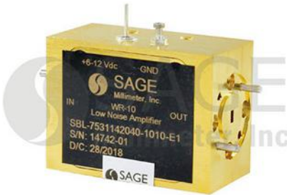
2. This LNA provides 20-dB gain and 4-dB noise figure from 75 to 110 GHz. (Courtesy of Sage Millimeter Inc.)
