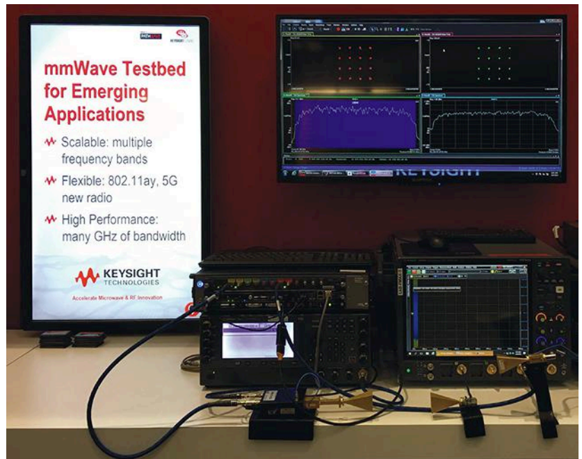
4. This is a wideband research-and-development mmWave test bed with a four-channel 110-GHz UXR.
