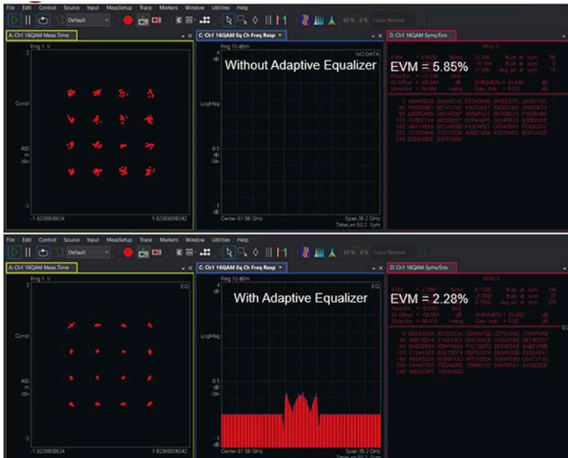
2. These simulation results with the added bandpass filter are given with and without adaptive equalization enabled.
