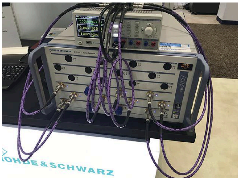
At IMS 2019, Rohde & Schwarz displayed this ZNBT40 multiport VNA, which covers a frequency range of 100 kHz to 40 GHz.
