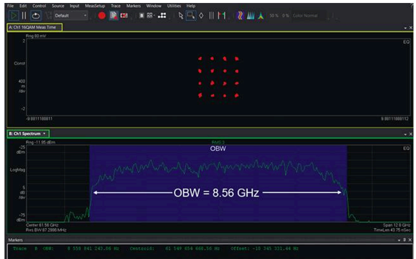
5. The UXR measurement revealed an OBW of 8.56 GHz.
