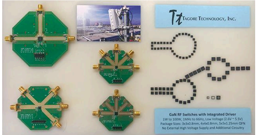
1. On display at IMS 2019 was Tagore Technology's family of GaN-based RF switches.
