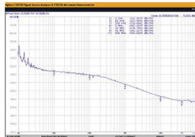
3. The low phase noise of the DFS2000 series dual frequency synthesizers combines with low harmonics and low spurious noise to deliver excellent spectral purity to 20 GHz. (Courtesy of FEI-Elcom Tech)
