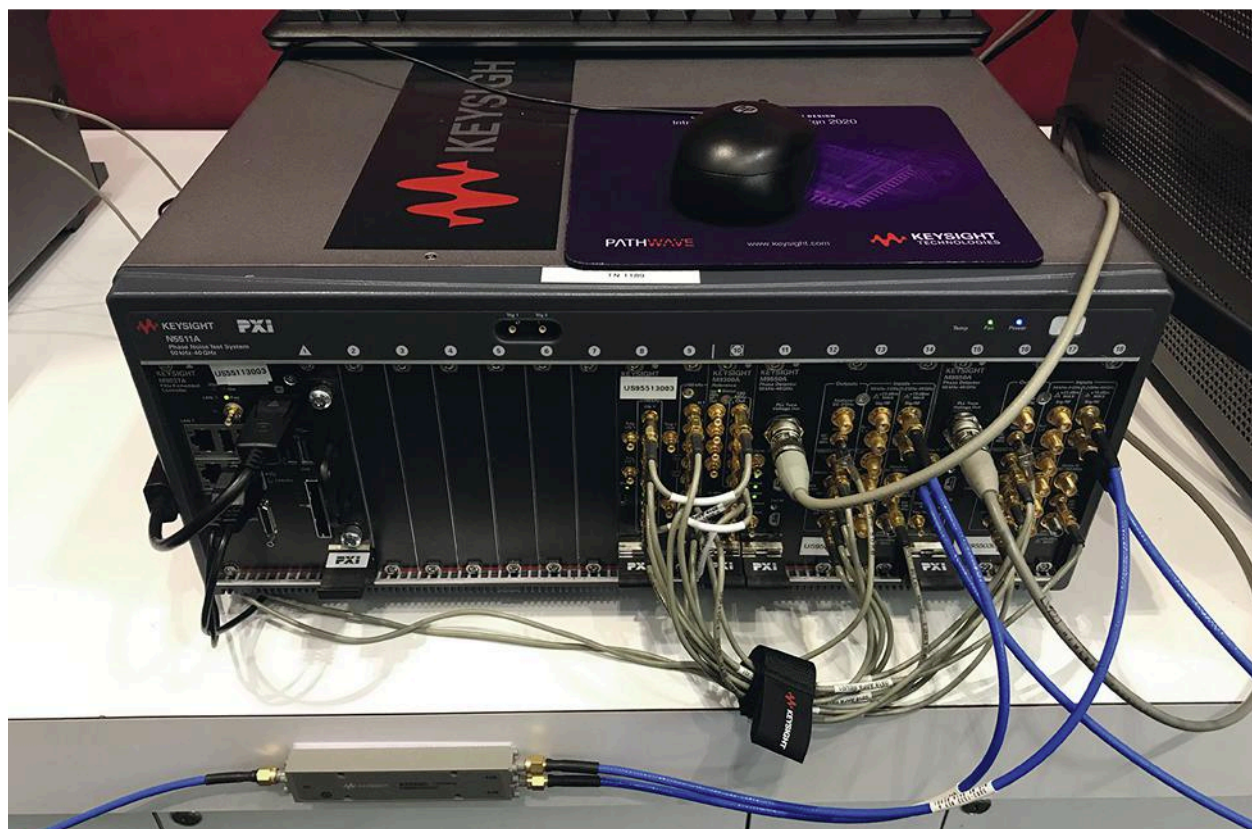
The N5511A phase-noise test system can measure phase noise down to -177 dBm/Hz.
