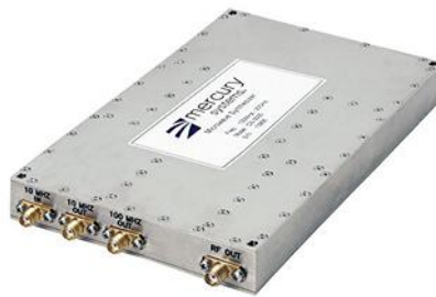
2. These compact modular frequency synthesizers are optimized for EW and ELINT systems. (Courtesy of Mercury Systems)
