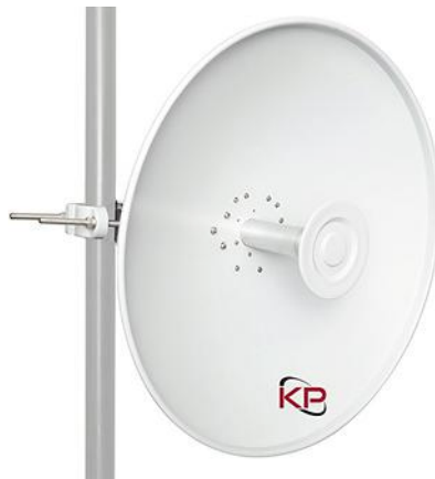
3. The KP-5PDN-2 2-ft. parabolic antenna covering 4.9 to 6.4 GHz has gain ranging from 27.5 to 29.8 dBi, depending on frequency. This increases the input power from a maximum of 50 W to an EIRP nearly 10 times that, enabling long distances to be covered.
