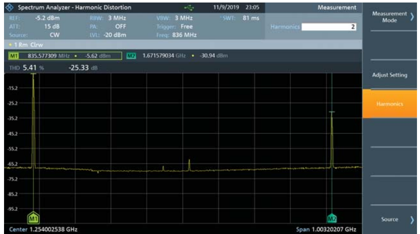
4. Thanks to the harmonic-distortion feature, the fundamental frequency and second-harmonic levels were easily determined.
