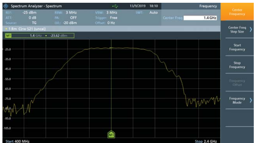
3. The built-in tracking generator makes it possible to perform scalar-network-analyzer measurements, such as this measurement of a bandpass filter with a center frequency of 1.4 GHz.
