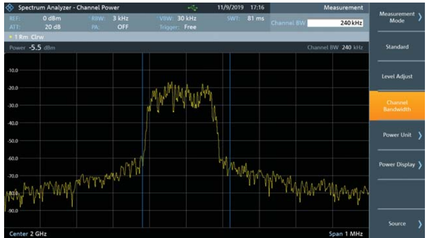
5. This screenshot shows a channel-power measurement of a 2-GHz QAM signal.
