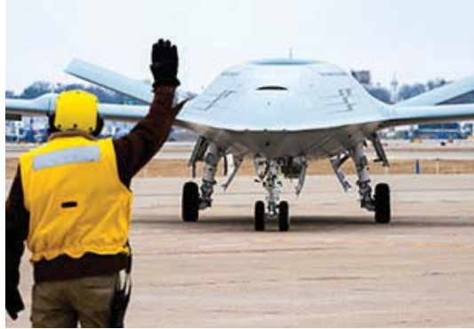
4. The MQ-25 UAV is being developed for the U.S. Navy for autonomous in-air refueling missions. (Courtesy of The Boeing Co.)
