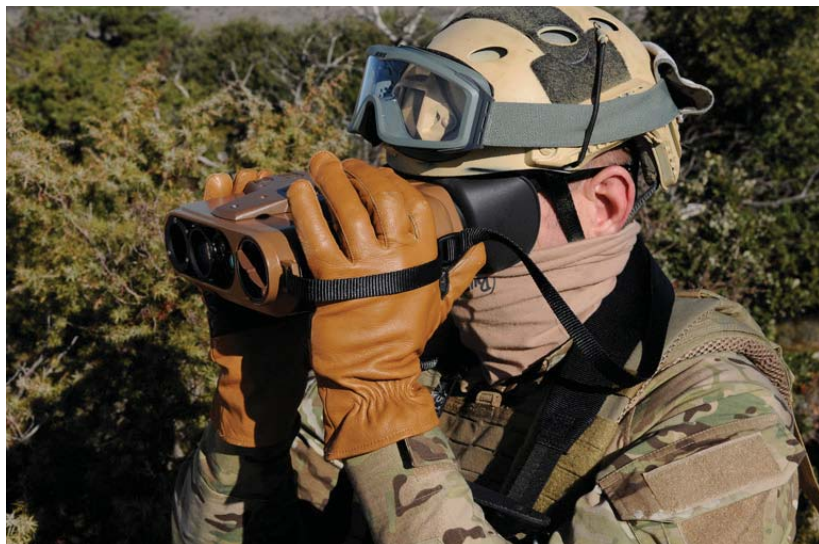
IR binoculars provide ground troops with enhanced night vision as well as wireless communications and laser range detection. (Courtesy of Safran Electronics & Defense)
