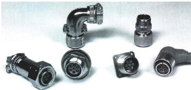
1. High-voltage connectors like the CMC-715 devices can be used to 15 kV dc at altitudes to 70,000 ft. and temperatures to +125°C.
