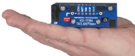
The compact TACLANE-Nano (KG-175N) network encryptor carries the NSA's TS/SCI certification for the most sensitive missions. (Courtesy of General Dynamics Mission Systems)
