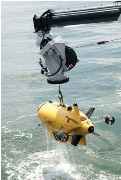
3. The Marlin is an autonomous underwater vehicle capable of performing inspections 1000 ft. beneath the surface of the water. (Courtesy of Lockheed Martin)
