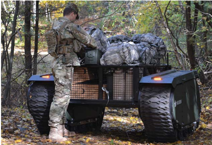
5. The Titan is a modular UGV that can be reconfigured as mission requirements change. (Courtesy of QinetiQ North America)
