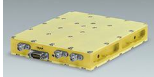
7. Many integrated subsystems will be on display at the 2016 IMS Exhibition, including this C-band transceiver with GaN-fired transmitter. (Courtesy of TRAK Microwave Corp.)
