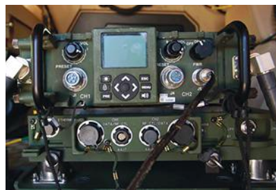
6. Mid-Tier Networking Vehicular Radios (MNVRs). MNVRs are vehicle-mounted modular radios designed for secure, short-range mobile communications on the battlefield. (Courtesy of Harris Corp.)
