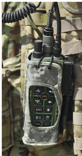
4. A Rifleman Radio operates to 1,850 MHz and includes a GPS receiver for position location. (Courtesy of General Dynamics)
