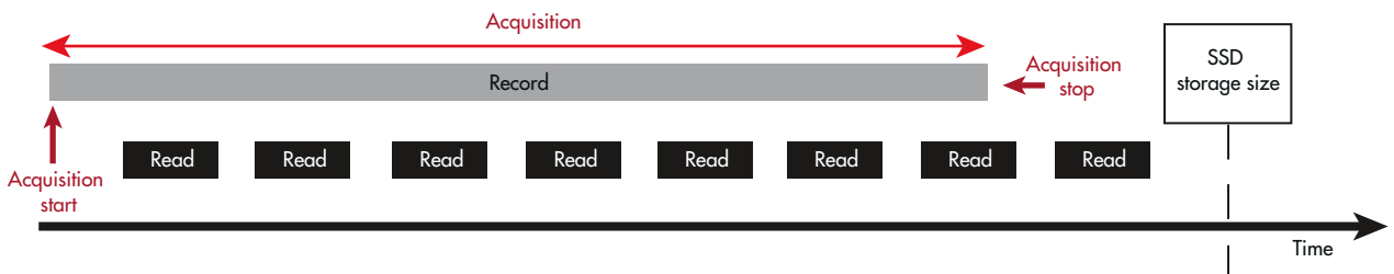
2. This is an example of a continuous signal-acquisition and readout approach showing gapless acquisition (no data loss). This system records signal-acquisition data from several hours to as long as several days at a time.
