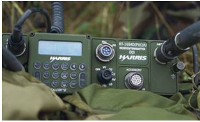
5. Operating at these lower frequencies (1.6 to 60 MHz), an AN/PRC-150(C) tactical radio provides reliable operation whether carried or mounted in a vehicle. (Courtesy of Harris Corp.)
