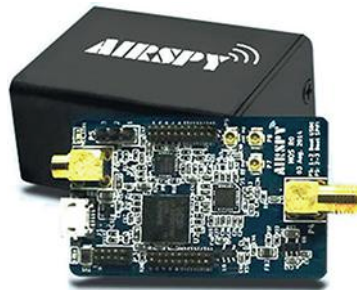
3. For those who need only receive functionality, the Airspy One series of SDRs offer continuous coverage from 24 to 1,800 MHz. (Photo courtesy of Airspy)
