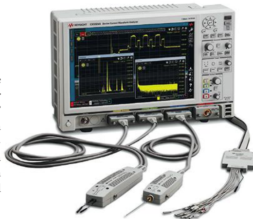
2. Three current sensors are available for the CX3300 series analyzers—models CX1101A, CX1102A, and CX1103A.
