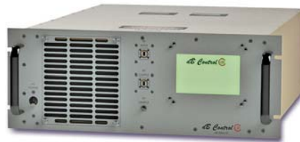
1. Model dB-3860-01 is a pulsed Ka-band TWTA with color-touchscreen local-control interface.
