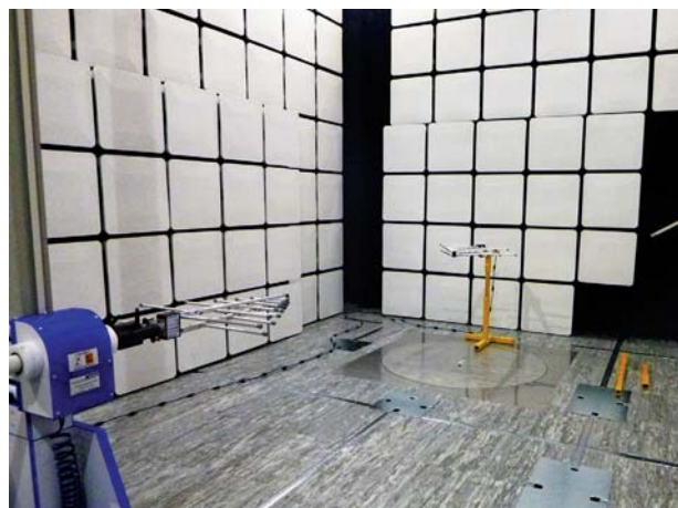
2. This is a CISPR-16-compliant 3m chamber lined with ULTRA UH series absorbers.
