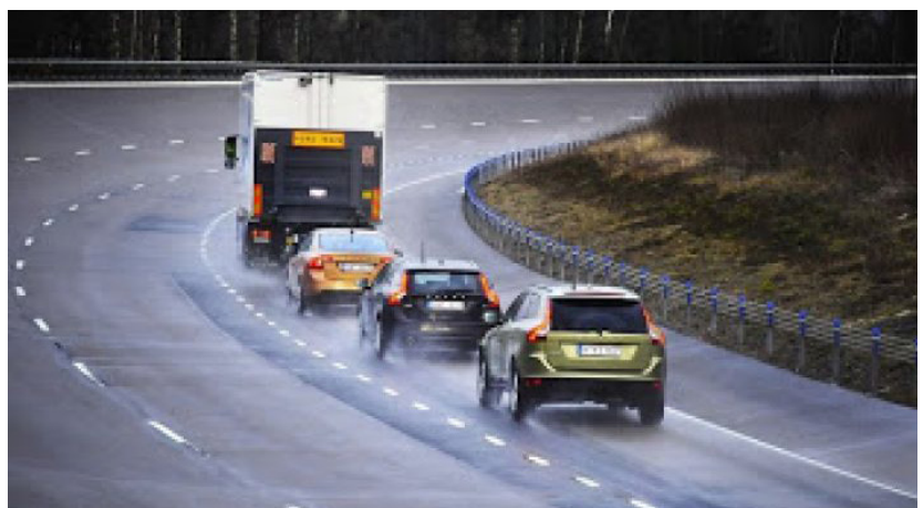
2. This dash-cam image captured four vehicles performing spontaneous platooning behind a large truck, which lowers wind resistance even further than an open formation. According to the driver who observed it, the car closest to the truck acted as sort of a "ring leader" by holding spaces open for the other vehicles to form the platoon before easing into position behind the truck. (Credit: Next Big Future)
