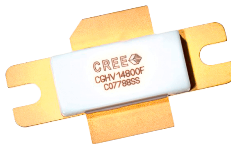
1. High-power GaN discrete transistors require rugged metal/ceramic packages to help dissipate heat, such as used with this L-band GaN-on-SiC transistor for L-band applications from 960 to 1400 MHz. (Courtesy of Wolfspeed/Cree)
