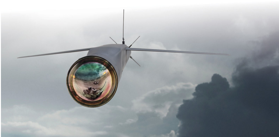
1. The StormBreaker autonomously detects and destroys moving targets in foul weather, using AI to comb through data collected by multiple seekers including millimeter-wave radar, IR imaging, and laser-based systems. (Courtesy of Raytheon Technologies, Raytheon Missiles & Defense)
