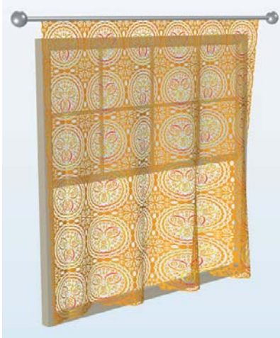
2. Shown is an imaginary view of a frequency-selective-surface curtain hanging in front of a window; this view was created using the COMSOL Multiphysics software.
