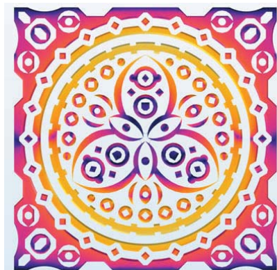
5. Shown is the electric-field distribution on the unit cell of the frequency-selective surface at 1.9 GHz.
