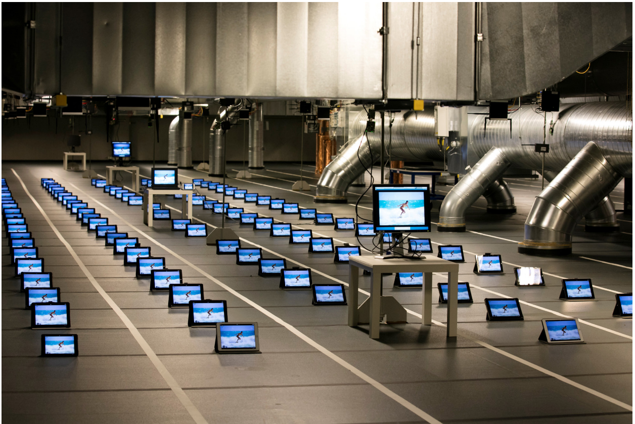
2. Shown is imec's (remote) IDLab test infrastructure, where all possible wireless technologies can be put to the test—from Wi-Fi to 4G, 5G, and even future 6G radio architectures based on distributed massive MIMO.
