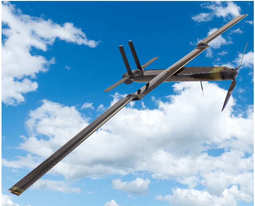
2. The Outrider, a compact UAS, can be launched from canisters that fit inside submarine missile tubes. (Courtesy of Lockheed Martin Corp.)
