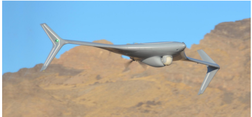
3. The Bat series of UAS devices are constructed with large wingspans to handle multiple EW sensor payloads. (Courtesy of Lockheed Martin Corp.)
