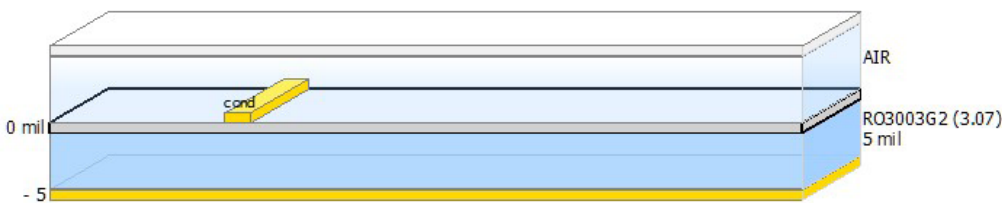
1. Shown is the layer stackup of a microstrip filter built on Rogers RO3003G2 PTFE laminate with a thickness of 127 µm.
