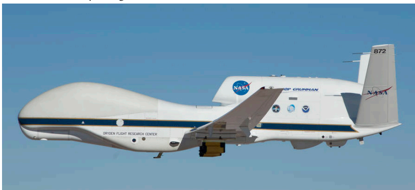
1. The Global Hawk is a high-altitude UAV that has shown the endurance to remain in flight for 30 hours continuously. (Courtesy of Northrop Grumman)
