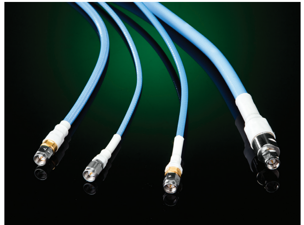
4. Standard PhaseTrack cables and cable assemblies incorporate a proprietary dielectric for high phase stability over temperature. A cable with 0.108-in. diameter has a cutoff frequency of 80 GHz. (Courtesy of Times Microwave Systems)
