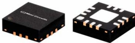
Mini-Circuits' model PMA3-83MP+ is a medium-power, monolithic surface-mount amplifier ideal for radar and communications applications from 0.4 to 8.0 GHz. It's capable of +27.8 dBm typical output power at 1-dB compression to 2 GHz and +25.3 dBm to 8.0 GHz. Noise figure is typically 3.5 dB across the full frequency range while full band gain is typically 17.3 dB. The RoHS-
