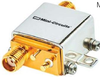
Mini-Circuits' model ZX60-06203ALN+ is a low-noise amplifier (LNA) with medium output power from 6 to 20 GHz. Gain is typically 17 dB through 20 GHz while noise figure is typically 2.2 dB to 12 GHz and 3.3 dB to 20 GHz. Suited for radios, radar, and EW, the RoHS-compliant LNA provides at least +14 dBm of output power at 1-dB compression. It measures 0.74 × 0.75 × 0.46 in. (18.80 × 19.10 × 11.68 mm) with female SMA connectors.
