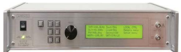
Avtech offers a full line of 100, 200, 500, 700 and 1000 Volt user-friendly pulsers capable of driving impedances of 50  $\Omega$  and higher. The **AVR Series** is suitable for semiconductor and laser diode characterization, time-of-flight applications, attenuator testing, and other applications requiring 10, 20, or 50 ns rise times, pulse widths from 100 ns to 100 us, and PRFs up to 100 kHz. GPIB, RS-232, and Ethernet ports are standard.
