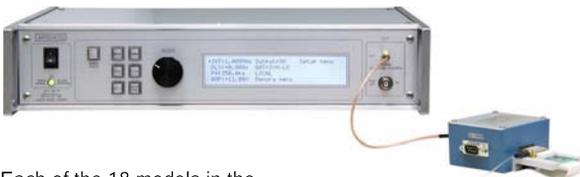
Each of the 18 models in the Avtech **AVO-9 Series** of pulsed laser diode drivers includes a replaceable output module with an ultra-high-speed socket, suitable for use with sub-nanosecond pulses.
