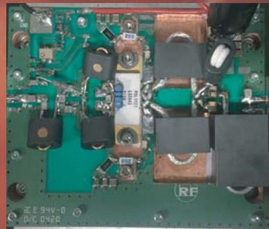
Pictured is the LS2641 transistor mounted in the TB263A evaluation amplifier; 250W CW, 30 - 512MHz, 36V, 20dB. Both available now.
