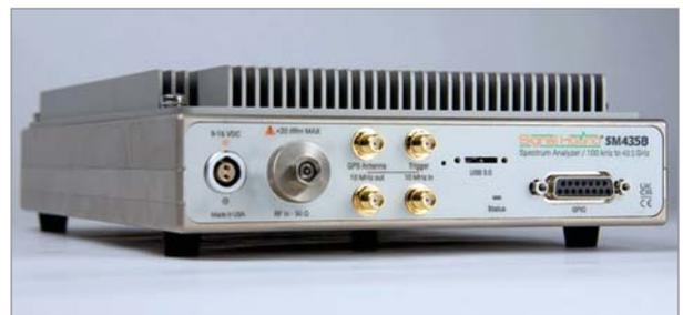
8. Signal Hound's latest spectrum analyzer and receiver combines 110-dB dynamic range, 1-THz sweep speed, and 160-MHz real-time bandwidth within a compact form factor.
