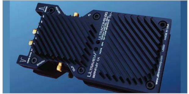
7. The Ultraview-8G comb generator offers a 10-MHz to 2-GHz picket for antenna range testing, communications, and jamming applications.
