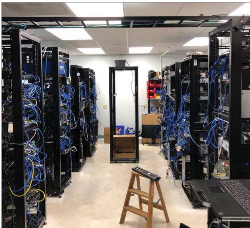
3. Green Hills Software's Embedded Board Farm allows remote developers to test real hardware.
