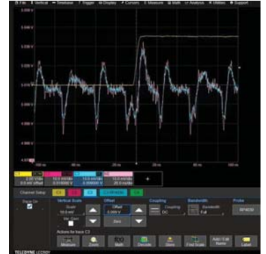
5. A rail probe (blue trace) offers a higher SNR than a 10x passive probe (red trace).
