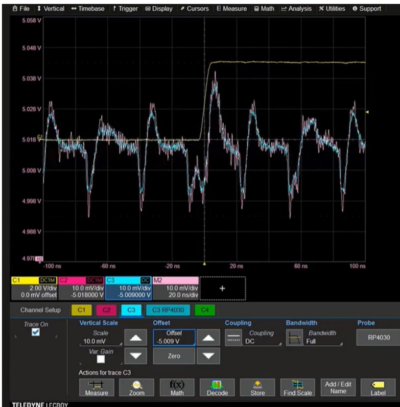
5. A rail probe (blue trace) offers a higher SNR than a 10x passive probe (red trace).
