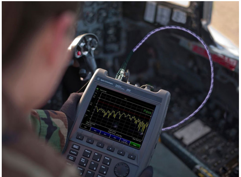
1. Shown is Keysight's FieldFox handheld analyzer connected with W.L. Gore's Phaseflex microwave/RF test assemblies used during flight-line testing. (Courtesy of Keysight Technologies)
