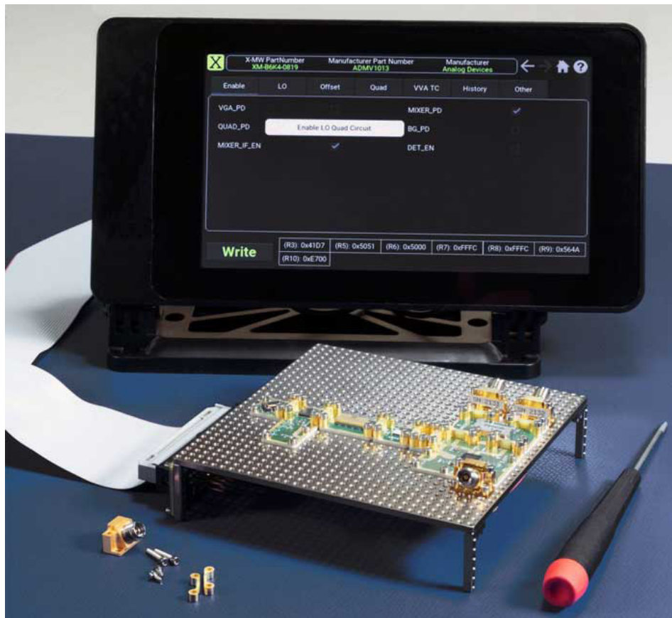
4. The XM-RDK-201/ADMV1013 frequency-upconversion kit from X-Microwave provides components needed for upconversion of RF signals to the range of 24 to 44 GHz.
