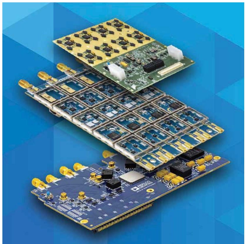
1. Analog Devices’ X-Band Phased Array Platform features high-speed mixed-signal ICs assembled on three PCBs and works with a fourth controller PCB for extensive phased-array beamforming experimentation.
