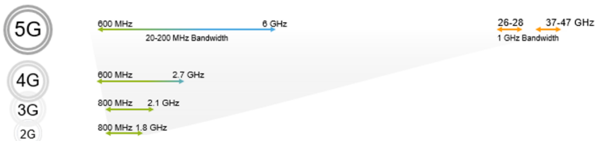
1. 5G adds new frequency spectrum, including the area between 2.7 and 6 GHz and a completely new part above 25 GHz.
