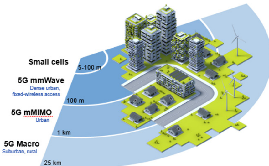
2. 5G densification brings capacity in layers.
