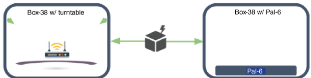
2. A basic test setup for TR-398 Issue 2 Wi-Fi performance testing.
