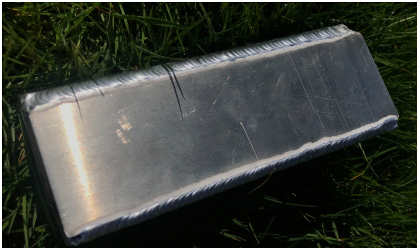
2: Organic welds produced by the OpenSource Direct from Solar Array TIG Welder.
