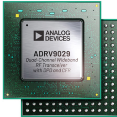
1. As an example of an SoC, this 75- to 6000-MHz agile transceiver is housed within a 289-ball, CSP_BGA package measuring 14 × 14 mm. (Courtesy of Analog Devices)
