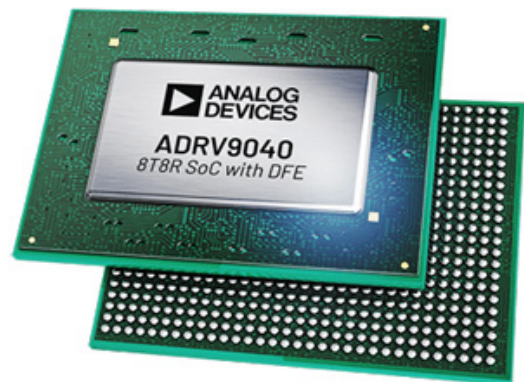
2. Though this is a larger SoC, coming in a 27 × 20 mm, 736-ball BGA housing, the transceiver has eight receivers and transmitters for 650 to 6000 MHz. (Courtesy of Analog Devices)
