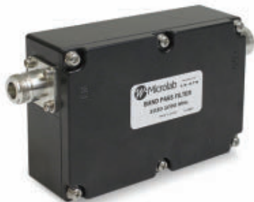
3. Coaxial bandpass filters in the LA-37N series target IFF applications from 1,030 to 1,090 MHz with passband power-handling capability of 100 W CW and 3 kW peak. Microlab/FXR
