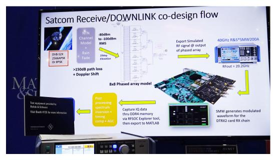
vendors' products to allow for RF/microwave-related design work. For example, the company demoed how <u>Otava's DTRX2 dual-transceiver mmWave radio card</u> can team with MathWorks tools to target satellite-communications development to RFSoCs, using the Otava product to conduct over-the-air testing (**Fig. 4**).
