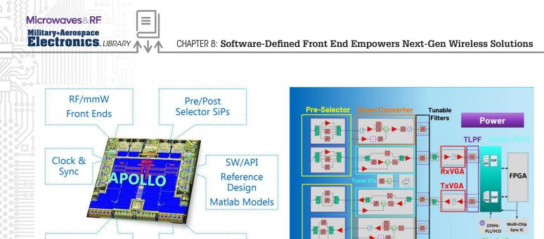
Features of the Apollo MxFE 4T4R include on-chip DSP, real-time FFT sniffer, full-rate programmable FIR filter, 128-tap complex FIR filter, fast-hopping NCOs, DDCs/DUCs, and fractional sample-rate converter.
