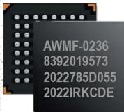
1. An example of the latest in beamforming ICs is Anokiwave's AWMF-0236, a quad-channel, dualpolarization device that covers 37 to 43.5 GHz.
