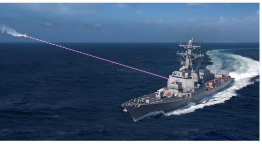
High Energy Laser and Integrated Optical-dazzler and Surveillance (HELIOS) system, a 60-kilowatt weapon developed by Lockheed Martin, was test launched on the destroyer USS Preble in August 2022.
