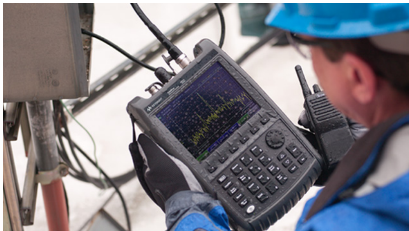
2. The FieldFox line of portable spectrum analyzers includes multifunction measurement tools with upper-frequency limits as high as 54 GHz in support of 5G wireless-network OTA testing. (Courtesy of Keysight Technology)
