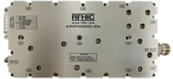
8. Built using on GaN-on-SiC technology, this SSPA from RHFIC provides 65 W output power from 2 to 6 GHz in a package measuring just 175 \times 90 \times 23 mm. (Courtesy of RHFIC)
