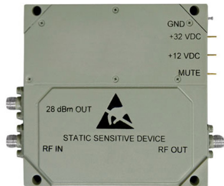
6. Designed for pulsed operation, Mercury's PA delivers as much as 1600-W saturated output power from 1.2 to 1.4 GHz. (Courtesy of Mercury Systems)
