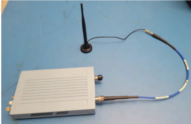
4. This is the measurement setup for a Wi-Fi antenna that receives and transmits in the 2.4-GHz band.
