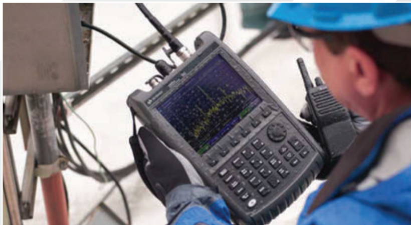
2. The FieldFox line of portable spectrum analyzers includes multifunction measurement tools with upper-frequency limits as high as 54 GHz in support of 5G wireless-network OTA testing. Keysight Technologies
