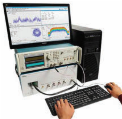
4. Portable RTSAs in the RSA7100A/B line offer acquisition bandwidths as wide as 800 MHz from 16 kHz to 26.5 GHz. Tektronix
