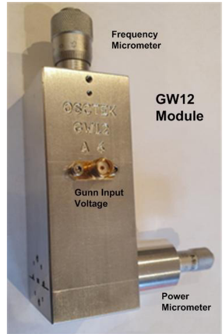
7. As shown, WR12 Gunn oscillators from Osctek are fitted for both cavity frequency adjustment power optimization.
