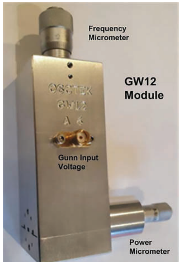
7. As shown, WR12 Gunn oscillators from Osctek are fitted for both cavity frequency adjustment power optimization.
