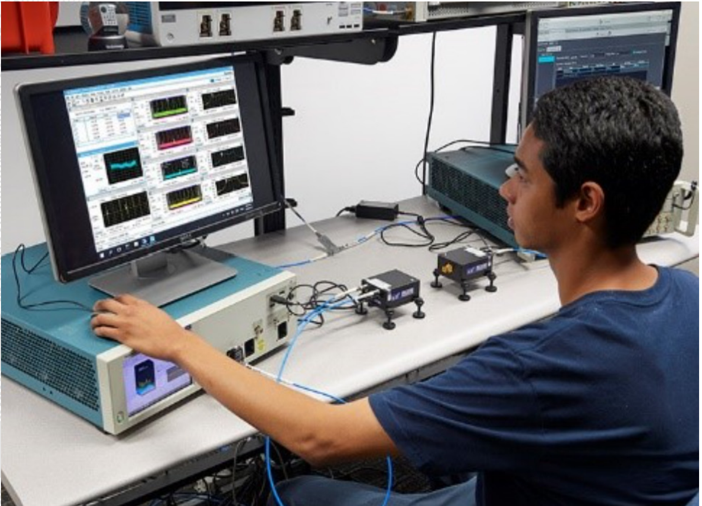
2. An RF engineer analyzes phase-coherent signals using SignalVu software. Tektronix
