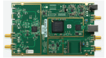
2. Model USRP B200 is an SDR/CR with one receive and one transmit channel on a single PCB powered by USB connection. Digilent
