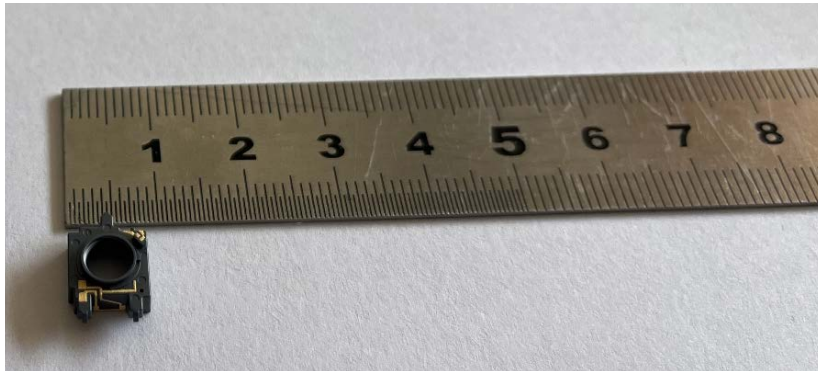
3. A Wi-Fi and Bluetooth LDS antenna fabricated with LCP material, as shown here, offers significant size reductions without degrading performance. (Photo by Chris Zhong)
