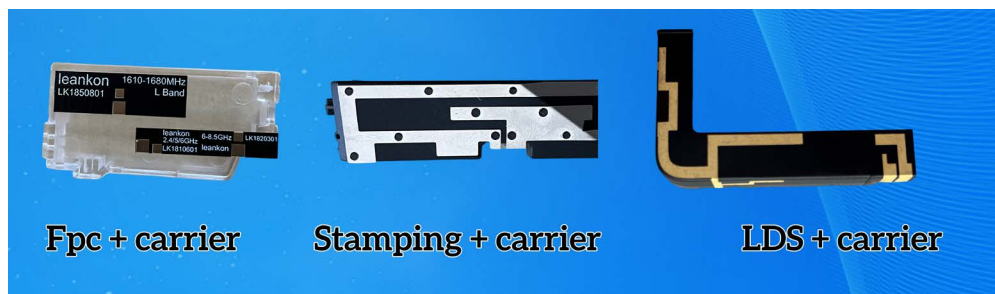
1. Shown are some antenna manufacturing processes: FPC on carrier, stamping on carrier, and LDS technologies. (Photo by Chris Zhong)
