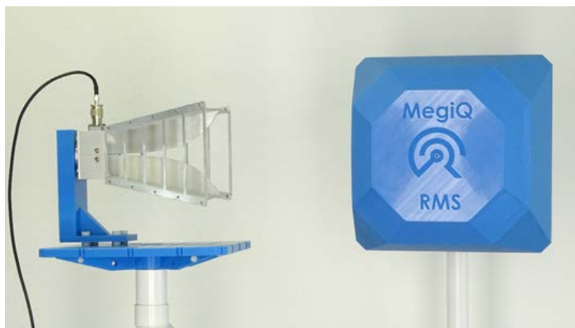
9. Shown here is MegiQ's RMS measuring a horn antenna.
